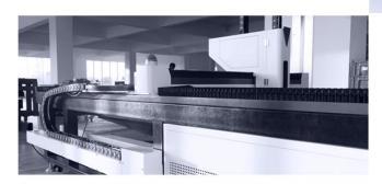
Gantry structure, imported high precision ballscrew transmission, running stable.
