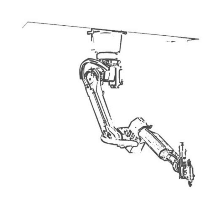
The machine can cut non-standard shape material. It can be six axis feed and is able to cut from 360 degree. Moreover, some non-standard materials, such as some with fixed geometry and angle, can also be cut by it.
